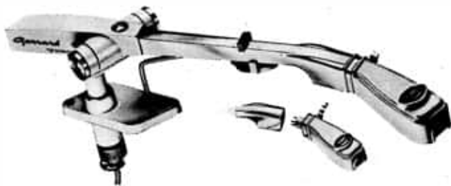
Garrard transcription pickup arm is adjustable for length, height, stylus angle and pressure. The Model TPA 10, as shown, is a monaural type.
