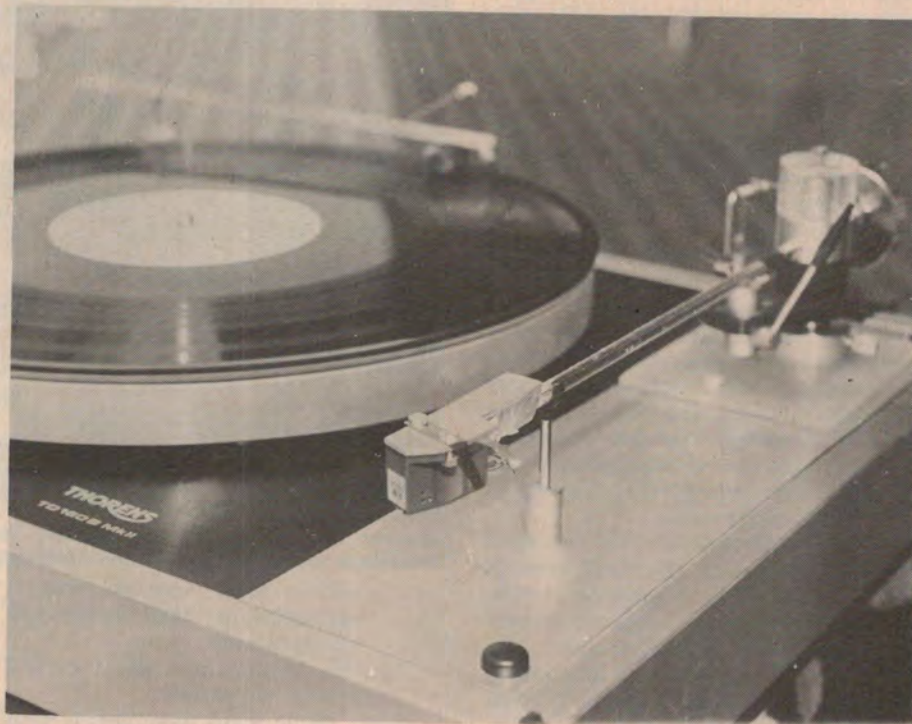
The revamped tone arm assembly mounted on my Thorens TD160 Mk II turntable
