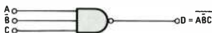
Fig. 10. In a NAND expression, the result of all ANDing is simply inverted.
