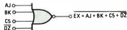
Fig. 11. Multiple-input NANDs do not need to have their variables separated by parentheses for clarity.
