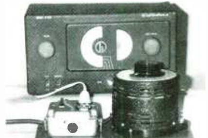
More than just a Christmas-tree bulb saver, the autotransformer is used here to uncover a failing part in an old relic—a Hallicrafters SX-38B shortwave receiver.
