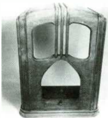
Shown here is the 7S232 now stripped of its finish. Much to my surprise and delight, the grain was not photographic, but really in the wood—just waiting to be brought out by an application of stain.
