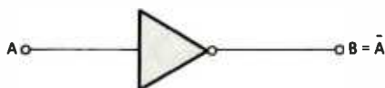
Fig. 6. The complement of a variable can be represented by placing a bar over that variable as shown here.
