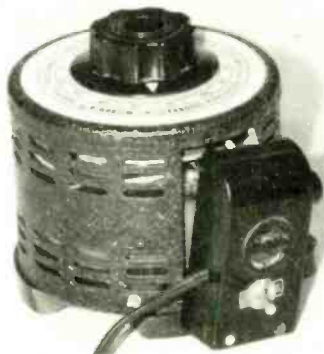
Here's the autotransformer ripe for repair. With a little effort, it turned out to be a worthwhile test-bench tool.
