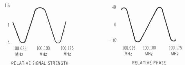
Fig. 3c—Amplitude and phase response of total transmission path containing one reflection.
