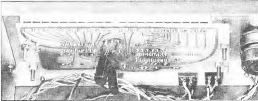
The back of the front! This shows the meter board mounting. Note the caps mounted on the rear of the board.
