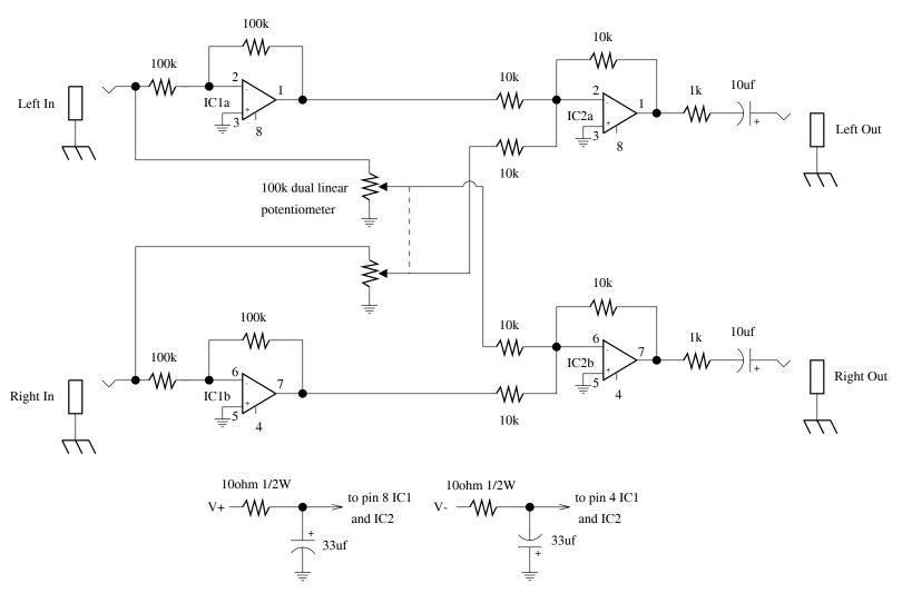
IC1 & IC2 are 5532 Dual Op amps for low noise. All resistors are 1% metal film 1/4W unless otherwise noted. Requires bipolar power supply from 9 to 15 volts.
