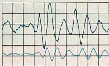
FIG. 3—SPECTRUM ANALYSIS of the "silent" groove of a record with considerable rumble. The upper curve is the input to the LFF, the lower curve is the output.
