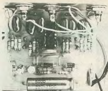
FIG. 11—THIS IS HOW the PC board should look when all components are in place on the board.
