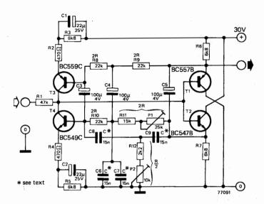
This filter will pass signals at its centre frequency while attenuating signals at all other frequencies.
