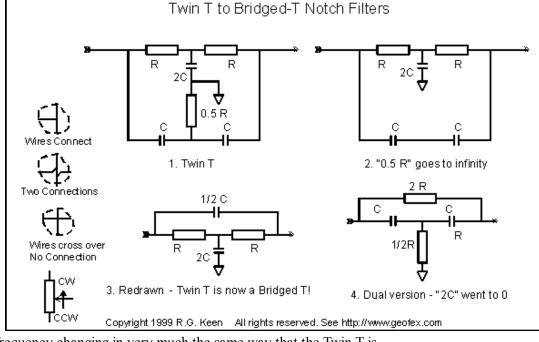
You've probably seen other RC filters used for scoops and notches. There are several of these, but one that comes up pretty often is the Bridged-T. This is a very close relative to the Twin T, as you can see from the sketch. If you take a basic Twin T and let the 0.5R leg resistance go to infinite resistance, and then combine the two series capacitors into one cap of 1/2 C, you get the Bridged-T. This thing is amenable to bootstrapping and
