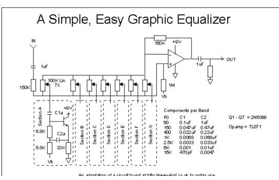
Here is a circuit diagram of a simple to build graphic EO. Notice that the circuit is very repetitious. the frequency selective elements are made of capacitors and "gyrators" that simulate the response of grounded inductors. These make the circuit free of real inductors, and are simpler to tune if tuning is needed. With standard value components, the frequency ranges come out a bit imperfect, but this is usually not noticeable in real
