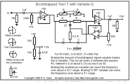
We can simply put a volume pot on the output of opamp U1b, leaving it just functioning as a buffer to keep the T unloaded, and use another opamp to drive the bootstrapping point of the T. This opamp is driven from the wiper of the pot, however. You can see that if the pot is fully up, the T is getting full bootstrapping for a Q of 50 or so, and when the pot is full down, the output of the second opamp is holding the
