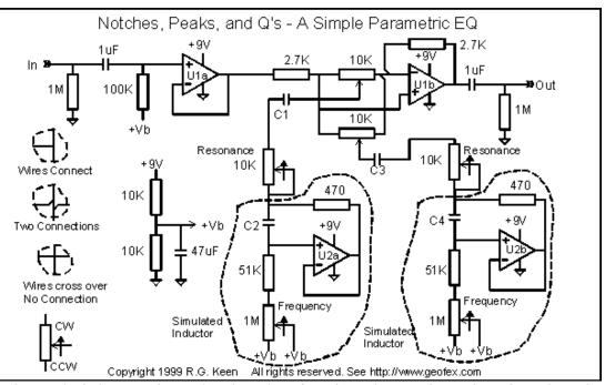
the first simulated inductor shown, the inductance is equal to the value of C2 times the 470 ohm resistor times the series resistance of the 51K and the setting of the 1M pot. Or more prosaicly, Leff = R1\*R2\*C, where R1=470, R2= series resistance, and C = C2's value.
