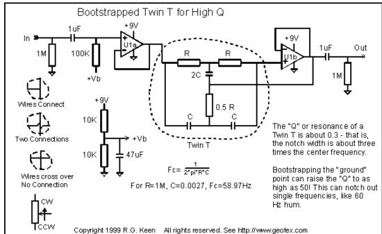
The section shown in the dotted line is a basic Twin T, if you ignore the opamps and connect the center junction of the 2C/0.5Rleg to ground. The twin T is one of the very few filters made from only resistors and capacitors that can cause an infinitely deep notch or attenuation. That is, at the exact center of the frequency dip it causes total attenuation of the signal.
