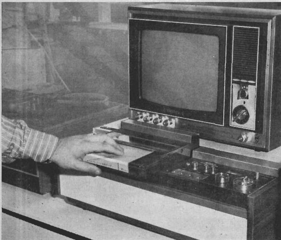
The Sony type VO-1700 video cassette recorder, using \frac{3}{4} inch tape, with a Trinitron colour receiver acting as a monitor.
