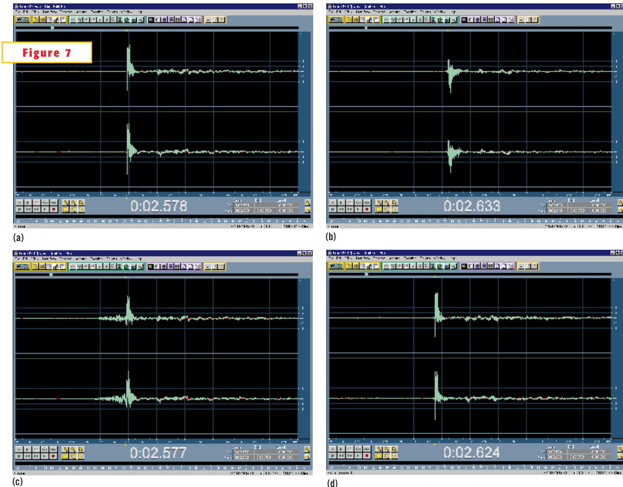
Oscilloscope (time-based) displays show the 15th transient in EBU SQAM file 27 (castanets), in original WAV (a) and lossy-compressed MP3 (b), RealAudio (c), and Windows Media Audio (d) formats.
