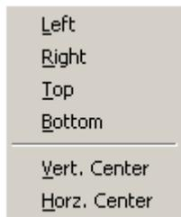
Align Objects provides Vertical Center & Horizontal Center functions, in addition to the Align Edges functions found on the Layout Toolbar.
