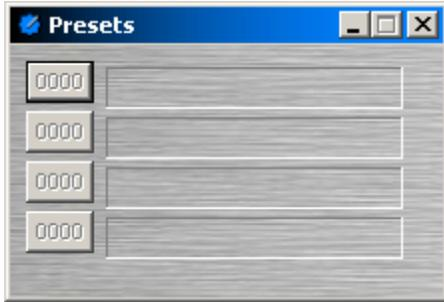
Right-clicking over a button provides a list of available Presets which can be assigned to that button. The Preset Number will appear on the button, and the Preset Name will appear to the right. Control Dialog Boxes for Preset Button components can be minimized to create user control surfaces (see Customizing Component Objects).
