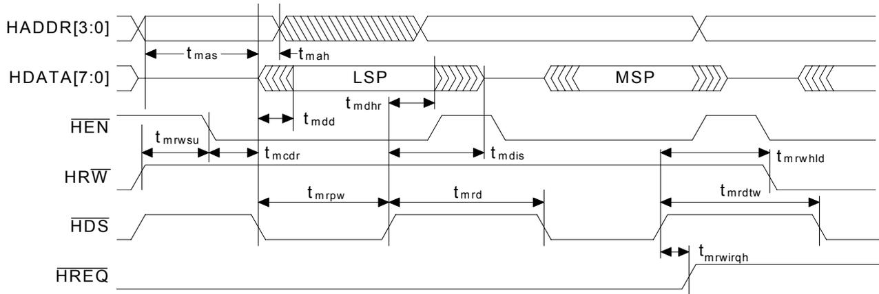
**Figure 14. Host Port Read Cycle Timing - Motorola Mode**
