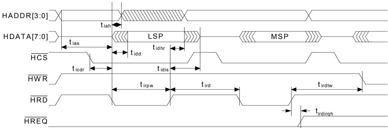
**Figure 16. Parallel Control Port - Intel Mode Read Cycle**
