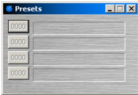
Remote Preset Buttons are identical to Preset Buttons, except they have control input nodes on the block. These control input nodes allow presets to be recalled via control output nodes on other component blocks. This provides remote control of preset selection, both from internal components and external controls. Control Dialog Boxes for Remote Preset Button components can be minimized to create user control surfaces (see Customizing Component Objects).
