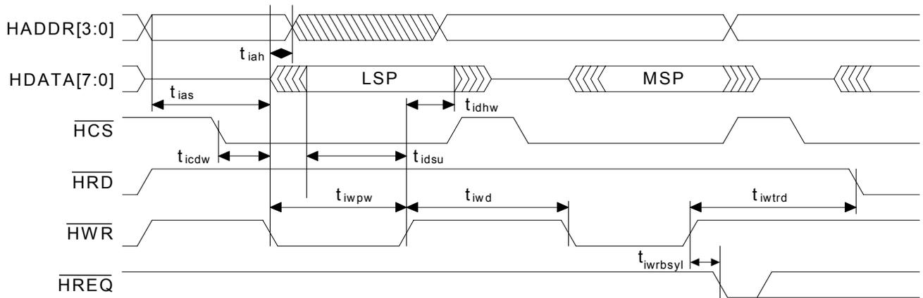
**Figure 17. Parallel Control Port - Intel Mode Write Cycle**
