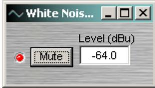
**Mute** turns on/off the generator. **Level** determines generator output level.
