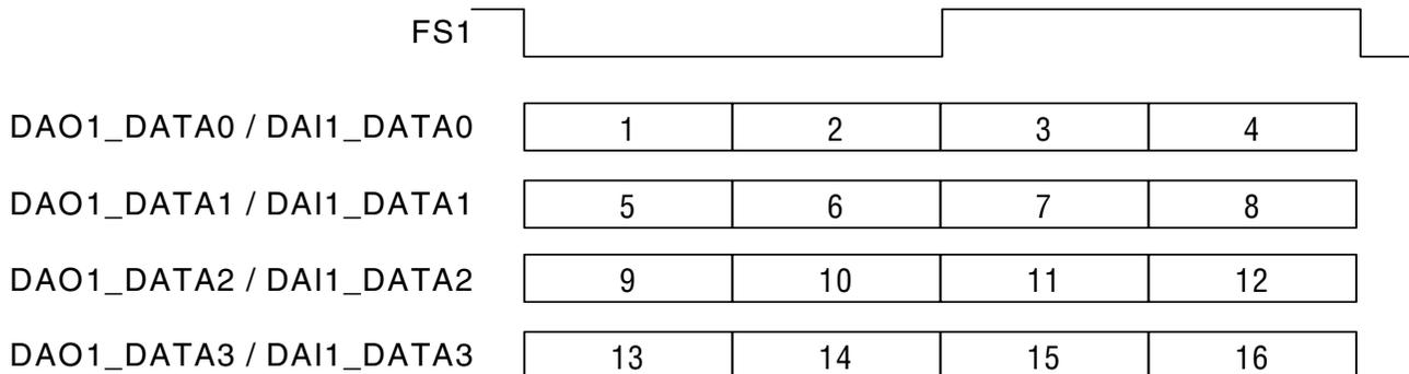
**Figure 5. Channel Structure for Synchronous Serial Audio at 128FS (One Sample Period) - CS18102x/CS49612x**
