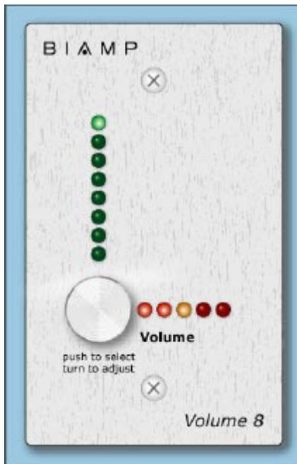
The Volume 8 is an external control device, which allows adjustment of eight selectable Audia volumes. Volumes can be individual or grouped levels within Audia. This includes Level Control blocks, as well as levels within other component blocks (such as Inputs/Outputs, Mixers, Equalizers, etc.).
