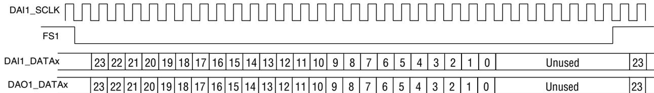
**Figure 10. Audio Data Timing Detail - I<sup>2</sup>S Mode, 64FS - CS18100x/CS49610x, CS18101x/CS49611x**
