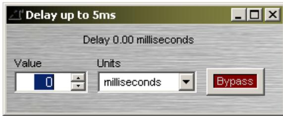
**Value** determines the amount of delay, based on the selected **Units**. **Units** selects either time (milliseconds) or distance (meters, centimeters, feet, or inches). **Bypass** disables the Delay without changing settings.
