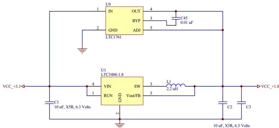
This is a simple switching regulator. It produces 1.8V at >500 mA at about 90% efficiency. A simple low drop out linear regulator would be a cheaper alternative at the expense of power. A linear regulator would dissipate about 0.75 watts max. This switching regulator dissipates about 0.10 watts max.
