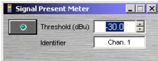
**Threshold** determines at what level the signal present indicator will light. **Identifier** provides a custom label, when dialog box is minimized (see below).
