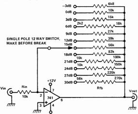
VOLTAGE GAIN = Rfb/Rin NOTE: AMPLIFIER INVERTS SIGNAL A handy little piece of test equipment is a preamplifier with stepped gain control selected by a rotary switch. The circuit here uses a single IC, a 741, 14 resistors and a single-pole, 12-way rotary switch.
