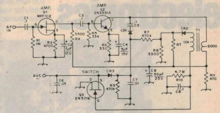
Like the original tube version, the AGC line must be of very high impedance. This would be the case with a FET IF system. If this circuit is to be used with an integrated circuit or bipolar IF amplifier system,
