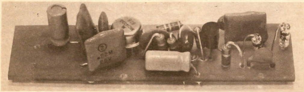
Fig. 4—Compressor is built on a printed-circuit board which just fits in mike case. Note that the electrolytic capacitor (white) in foreground is folded flat to board. Leave capacitor's leads a trifle long so it can be folded this way. Output of compressor is at left. Circuit's input is at the right.
