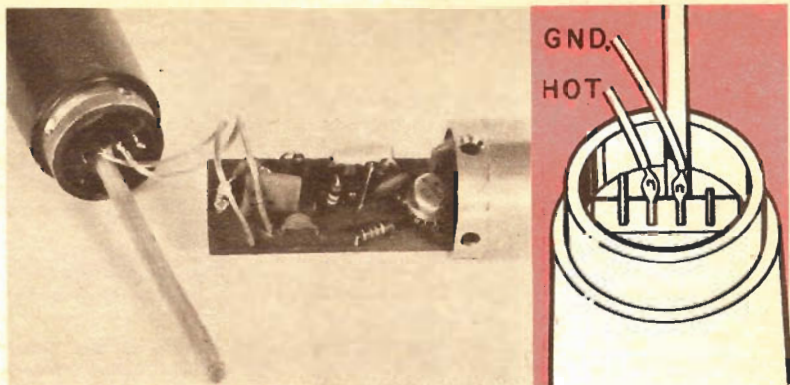
Fig. 5—Hollow tube sticking out of back of front half of mike is air-pressure relief tube for mike element. Tube slips under board during final assembly; don't damage it. Sketch at right shows connections to lugs in mike.
