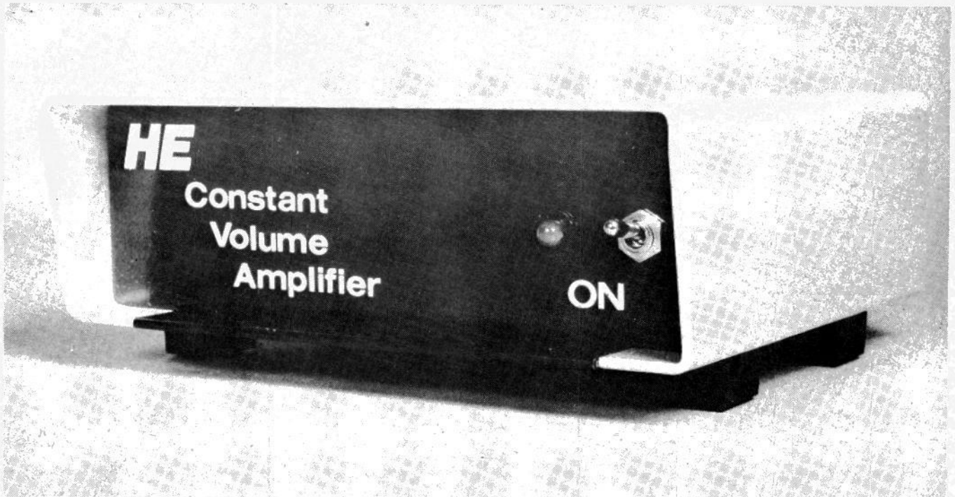
The on-off switch and LED keep the front panel neat and uncluttered.
