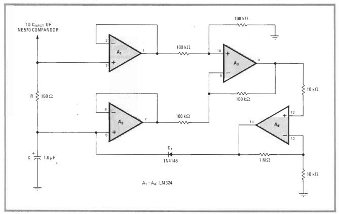
**Dynamic.** Circuit for decreasing NE570's attack time for large signals uses a quad operational amplifier for quick charging of compandor's averaging capacitor, C, in this way reducing its effective value. The fundamental waveform distortion from the compandor output is substantially reduced as a result, but third-harmonic distortion for low- and medium-amplitude signals is not substantially increased.
