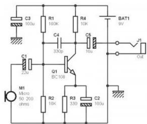
The microphone preamp based transistor described here is powered by 9 V and less than 1 mA current consumption, it will allows you to use a small 9 V rectangular conventional battery for several hours.
