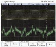
The distortion residual of the amplifier output at 1W with both channels driven into an 8D load [green] compared to the output itself [vellow]. As you can see, it is mainly a combination of 50 Hz, 100 Hz and even order harmonics of these frequencies, indicating that it's due to hum pick-up from the power supply. The actual distortion products at 2kHz and above can be seen superimposed on this waveform at a much lower level.
