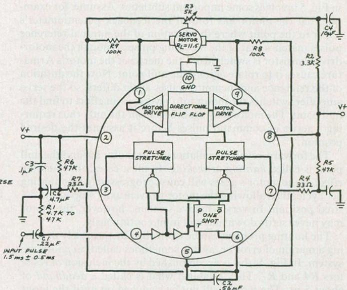
Fig. 5. Block diagram of NE543 servo amplifier.
