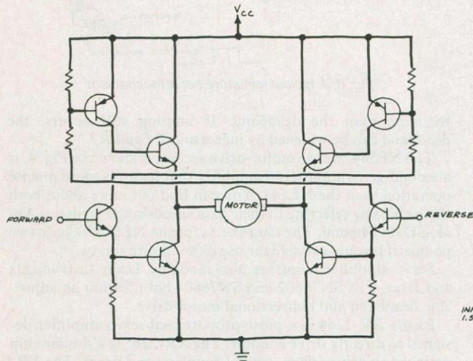
Fig. 4. Motor control circuit in Signetics NE544.
