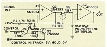
The low input current and high slew rate of the AD503J make it an excellent device for track-hold applications. This circuit will track a ±10V input signal at frequencies up to 4kHz. When the control input changes from Track (+5V) to Hold (0V), the series FET switch, Q3, opens, and the input signal voltage is retained on capacitor C1. The output amplifier, A2, provides a high input impedance to keep C1 from discharging too rapidly.
