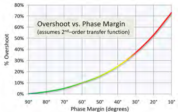
Figure 39: A 20-percent overshoot indicates approximately 45° phase margin—often considered to be satisfactory for most circuits.
