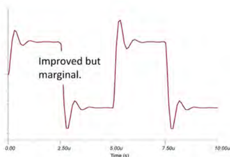
Figure 34: Using an op amp in a higher gain of 10 decreases the bandwidth of the closed-loop amplifier; however, the improvement is marginal.
