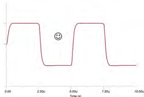
Figure 35: Using the same configuration, adding a C_c of 12 pF in parallel with the feedback resistor produces an ideal response.
