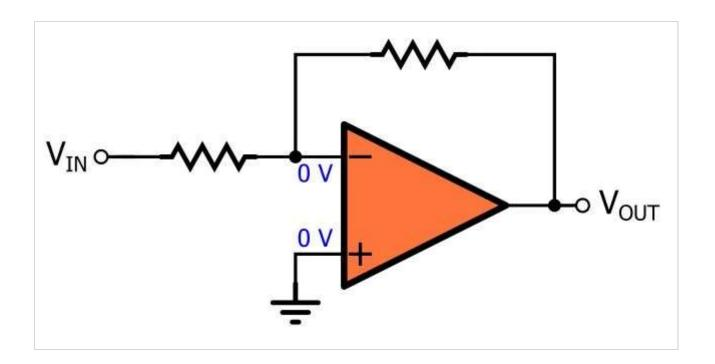
The standard method of obtaining an expression for the gain of this circuit is to assume that the voltage at the noninverting input terminal  $(V_{IN+})$  is equal to the voltage at the inverting terminal  $(V_{IN-})$ . Since the noninverting input terminal is grounded,  $V_{IN+} = 0$  V and thus  $V_{IN-} = 0$  V. But why? Why can we assume that two different voltages are the same?
