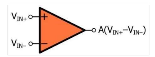
$$V_{OUT} = A imes (V_{IN+} - V_{IN-})$$
