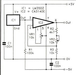
Fig. 1. Circuit diagram for the Improved Temperature Sensor Interface
