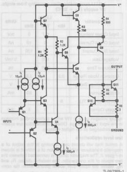
Figure 1. Simplified schematic of the comparator
