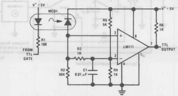
Figure 7. Data transmission system with near-infinite ground isolation
