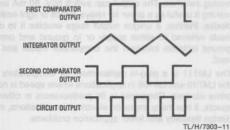
Figure 11. Waveforms for the frequency doubler
