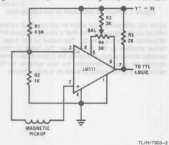
Figure 2. Zero crossing detector for magnetic transducer
