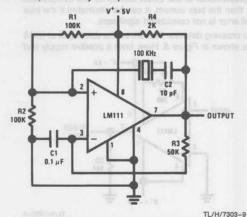
Figure 9. Crystal-controlled oscillator
