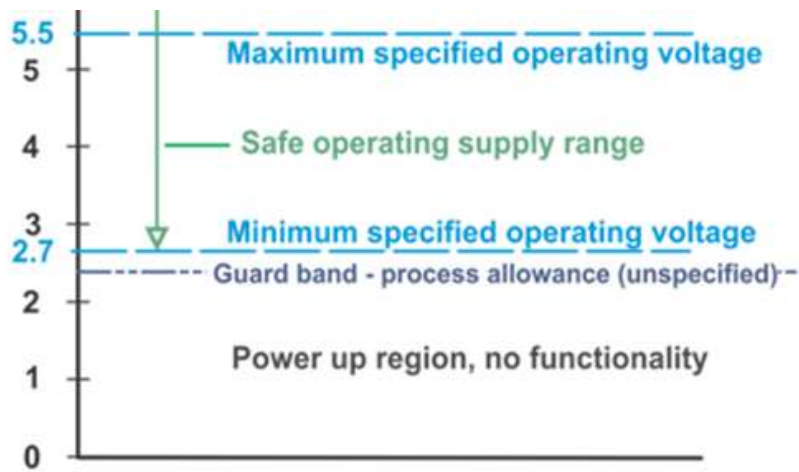
Figure 1: An example of the low operating voltage end for a CMOS op amp
