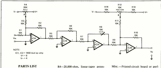
IC1, IC2—1458 dual op amp (see text) R1, R2, R3, R5, R6, R7, R9, R10, R11— 10,000-ohm, <sup>1</sup>/<sub>4</sub>-watt, 10% tolerance resistor
