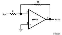
$$V_{OUT} = -\frac{R2}{R1}V_{IN}$$
