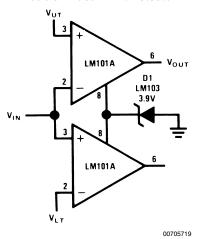
$$\begin{split} &V_{OUT}=4.6 \text{V for } V_{LT} \leq V_{IN} \leq V_{UT} \\ &V_{OUT}=0 \text{V for } V_{IN} < V_{LT} \text{ or } V_{IN} > V_{UT} \end{split}$$
