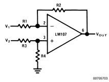
$$\begin{split} V_{OUT} &= \left(\frac{R1 + R2}{R3 + R4}\right) \frac{R4}{R1} V_2 - \frac{R2}{R1} V_1 \\ \text{For R1} &= R3 \text{ and } R2 = R4 \\ V_{OUT} &= \frac{R2}{R1} (V_2 - V_1) \\ R1//R2 &= R3//R4 \end{split}$$
