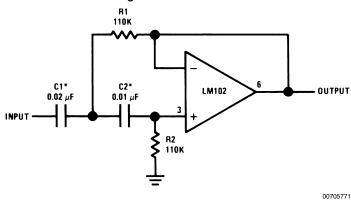
\*Values are for 100 Hz cutoff. Use metalized polycarbonate capacitors for good temperature stability.
