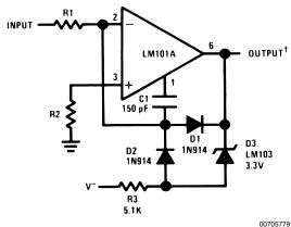
Propagation delay approximately 200 ns †DTL or TTL fanout of three. Minimize stray capacitance Pin 8
