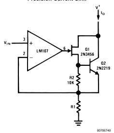
$I_{O} = \frac{V_{IN}}{R1}$  $V_{IN} \ge 0V$
