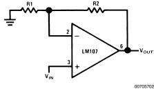
$$V_{OUT} = \frac{R1 + R2}{R1} V_{IN}$$
