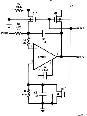
$^*Q1$  and Q3 should not have internal gate-protection diodes. Worst case drift less than 500  $\mu V/sec$  over  $-55^\circ C$  to  $+125^\circ C.$
