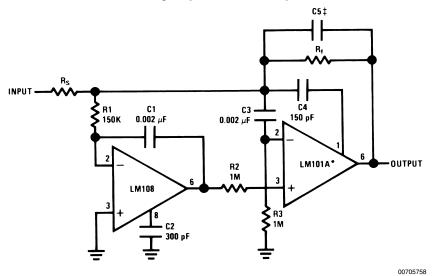
\*In addition to increasing speed, the LM101A raises high and low frequency gain, increases output drive capability and eliminates thermal feedback.
