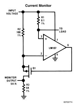
$V_{OUT} = \frac{R1\ R3}{R2}\,I_L$
