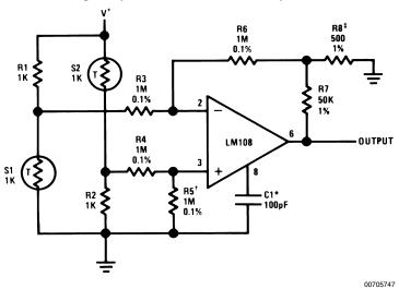
\*Reduces feed through of power supply noise by 20 dB and makes supply bypassing unnecessary.
