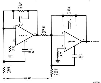
$\dagger \text{Matching determines common mode rejection.}$
