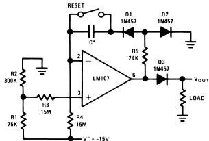
\*Low leakage  $-0.017~\mu F$  per second delay
