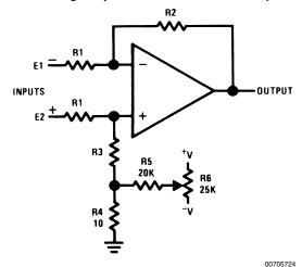
$$\begin{aligned} &R2 = R3 + R4 \\ &RANGE = \pm V \left(\frac{R5}{R4}\right) \left(\frac{R1}{R1 + R3}\right) \\ &GAIN = \frac{R2}{R1} \end{aligned}$$
