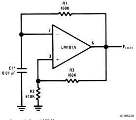
\*Chosen for oscillation at 100 Hz
