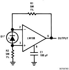
$V_{OUT} = 10 \text{ V/}\mu\text{A}$
