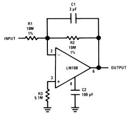
\*Source Impedance less than 100k gives less than 1% gain error.
