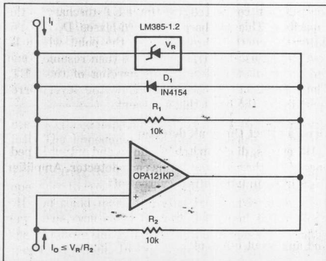
**Fig 6—A voltage reference in the feedback of this current inverter can clamp the output current to a level set by the voltage reference.**
