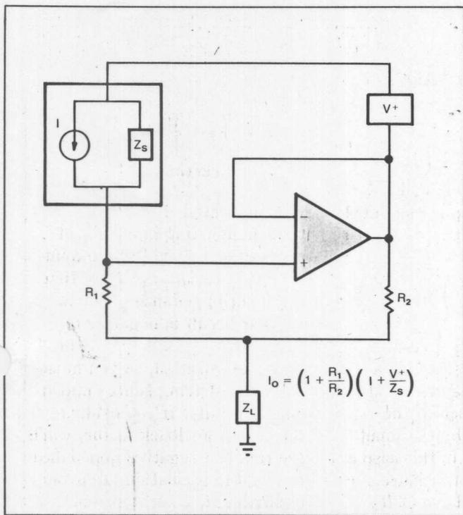
Fig 4—Driving the source's power-supply common from the op amp's output removes impedance loading errors from the noninverting current connection.
