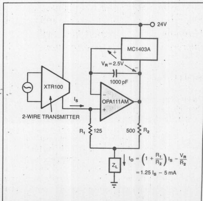
**Fig 3**—A voltage reference in a noninverting amplifier circuit develops a cancellation current that removes the output offset of a 2-wire transmitter.
