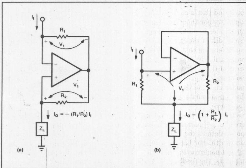
**Fig A**—These op-amp circuits amplify current instead of voltage. However, both the inverting (a) and the noninverting (b) current-mode configurations parallel similar voltage-amplifier designs.
