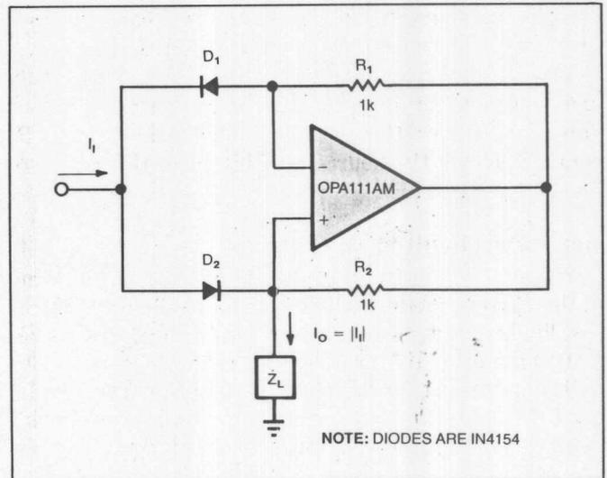
**Fig 7—The ease with which currents switch diodes simplifies absolute-value conversion in the current mode.**
