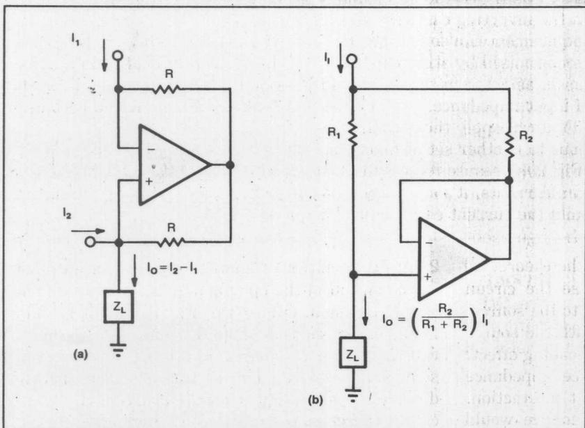
**Fig B**—Shifting connections in Fig A's circuits produce current amplifiers that are equivalent to difference amplifiers (a) and that can attenuate current (b).
