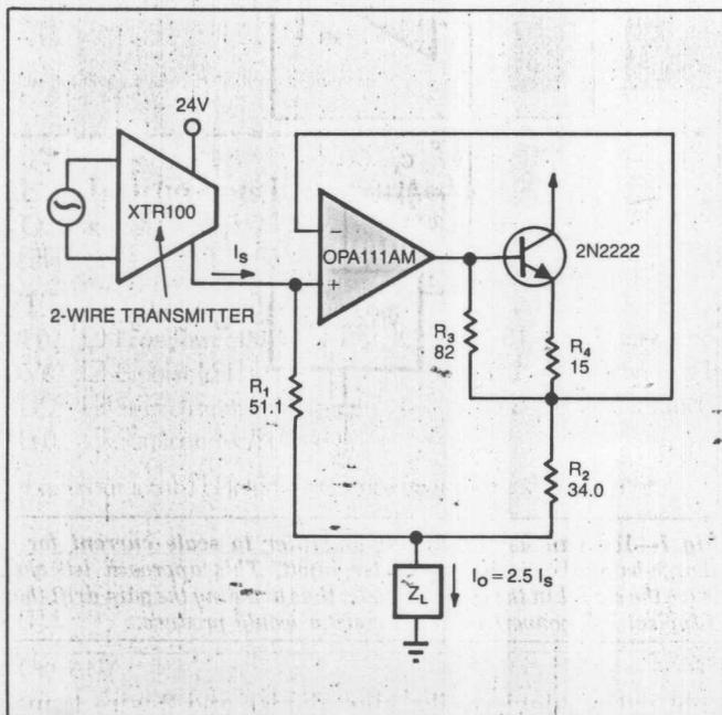
**Fig 2**—By boosting the op-amp output current, a noninverting current amplifier can raise the 4- to 20-mA output of a 2-wire transmitter to the 10- to 50-mA scale.
