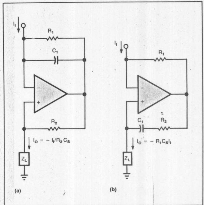
Fig 8—These designs translate integration (a) and differentiation (b) into current-mode functions from their voltage-mode counterparts.
