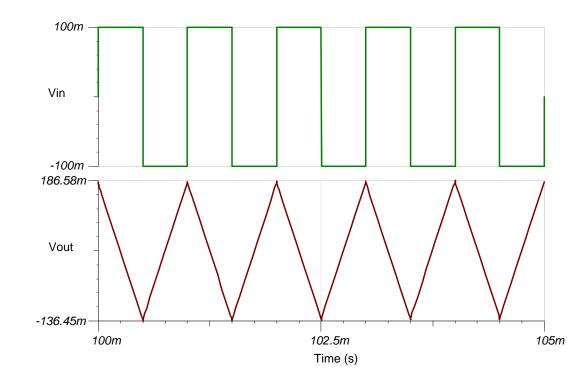
A 1-kHz square wave input yields a 1-kHz triangle wave output.
