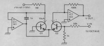
has a high temperature coefficient (-1.9 mV/°C) and so the reason for using a matched pair is to use the first transistor, Q1, to provide temperature compensation for the second.
