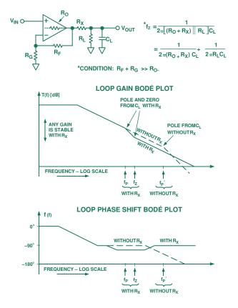
transfer function of the feedback network, thereby reducing the loop phase shift at high frequencies.
