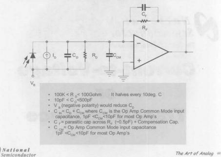
There are many applications which use photo diode to detect the intensity of the incident light. Examples would be: Barcode scanners, light meters, fiber optic receivers, industrial sensors, etc. The diode has a nearly linear output current for a very large range of light intensity. The voltage across the diode is held constant in order to minimize non-linearities.
