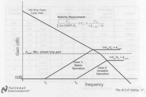
Devices which have a minimum closed loop gain requirement (i.e. LMH6624 & LMH6626) need special considerations when it comes to stability. These devices are optimized to provide maximum possible speed for the amount of power they use. In the case of the LMH6624 & LMH6626, the minimum closed loop configuration is 10V/V (20dB). In the I-V converter configuration, there is the additional constraint of increasing Noise Gain which gives rise to further phase shift which must be accounted for.
