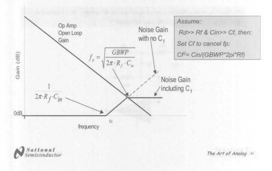
One interesting aspect of this type of amplifiers, also know as I-V converters, is that in almost all cases the frequency response needs to "shaped" or otherwise the circuit will oscillate. The high capacitance of the diode (including the op amp input capacitance), along with large Rf needed to get reasonable trans-impedance gain, will create enough phase shift around the loop that necessitates steps be taken to avoid oscillations.
