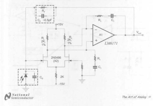
As we found earlier, the input noise current could have a profound effect on overall noise, especially with large Rf. Here is a neat way to optimize the I-V converter.
