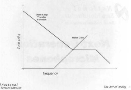
The composite amplifier just discussed could be made to have an open loop response resembling that shown here by the proper selection of R1, and C1. As can be observed on this plot, the noise gain and the X curves intersect each other at a point where the phase shift around the loop is 135 degrees (Phase margin of 45 degrees). Note that the useable BW did not have to be sacrificed to ensure adequate phase margin in this case.
