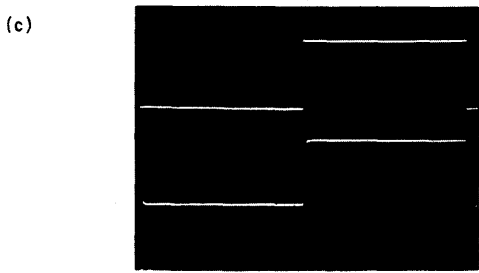
TOP TRACE: INPUT - 5V/DIV - 100 μsec/DIV BOTTOM TRACE: OUTPUT - SAME SCALE
