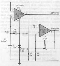
Figure 1. Self-Buffered Micropower Reference
