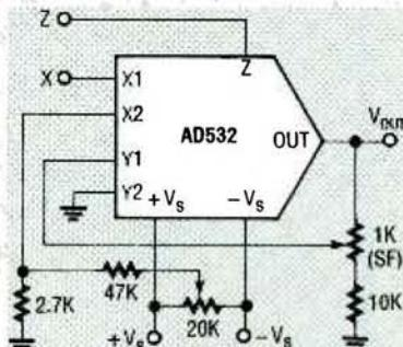
FIG. 12—SCHEMATIC DIAGRAM of the AD532 organized as a divider.
