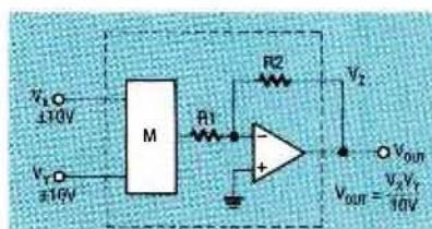
FIG. 3—MULTIPLIER IC CONNECTED as a multiplier.
