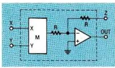
FIG. 1—FUNCTIONAL BLOCK DIAGRAM of a typical multiplier/divider.
