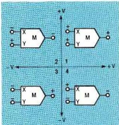
FIG. 2—DIAGRAM OF FOUR quadrants for multiplier shows how output polarity relates to input polarities.
