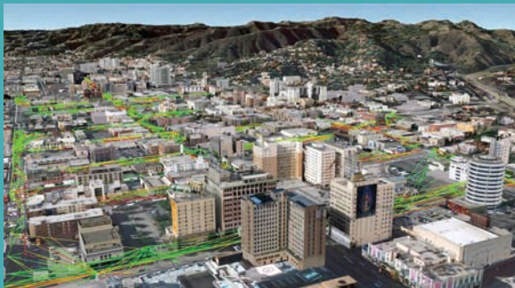
Figure A Streetline Networks' smart-parking management solution uses Linear Technology/Dust Networks' wireless technology in a wireless mesh network overlaid on urban streets. Wireless sensors buried in the pavement gather information on parking-space availability that is sent wirelessly to smartphone users.
