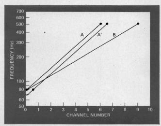
against the number of that stage, is linear. Therefore the frequency of the first stage can be plotted at abscissa zero, the frequency of the last stage can be plotted at abscissa (N – 1) where N is the total number of stages in the filter, and when the two points are connected by a straight line, the frequencies of all intermediate stages can then be read at a glance.
