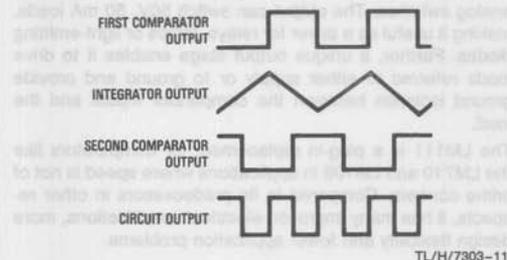
**Figure 11. Waveforms for the frequency doubler**
