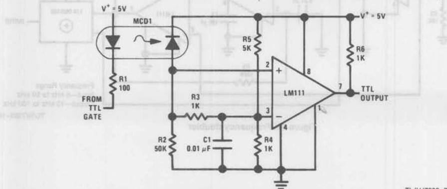
Figure 7. Data transmission system with near-infinite ground isolation
