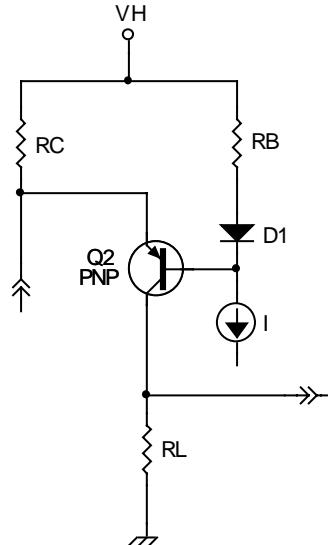
tracks variation in  $V_{BE}(Q2)$  with temperature, to a first approximation.  $R_B \cdot I$  sets the voltage across  $R_C$ , which provides current for both the translator collector and Q2. To minimize thermal distortion, this current should be split about equally between transistors, though to effect the low-end output voltage, Q1 will have to sink the total current.
