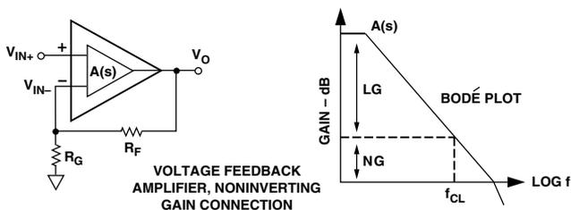
that no current flows into the op amp (infinite input impedance); both inputs will be at about the same potential (negative feedback and high open-loop gain)).
