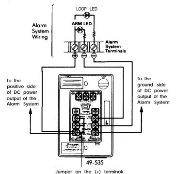
If your system has common negative (-) connections for its indicators, move the jumper to the negative ARM, LOOP, and POWER terminals and make connections similar to the drawing below.
