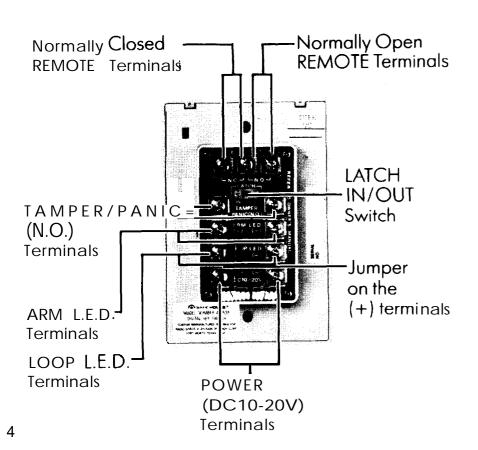
REMOTE Normally Open/Normally Closed Terminals - connect the appropriate pair of these terminals (N.O. or N.C.) to the remote arm/disarm terminals on your alarm; consult the manual for your system. The center terminal is a common connection for both N.O. and N.C. arm/disarm switches.
