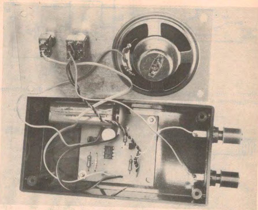
Here is a view of the works. The speaker is attached with contact adhesive.
