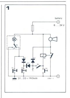
Figure 1. Circuit of the simplest burglar alarm consisting of three diodes and a switch. The door containing  $S_1$  is not protected. Additional door switches should be wired in parallel with  $S_2$ , other switches such as boot and glove compartment between point A' and earth.
