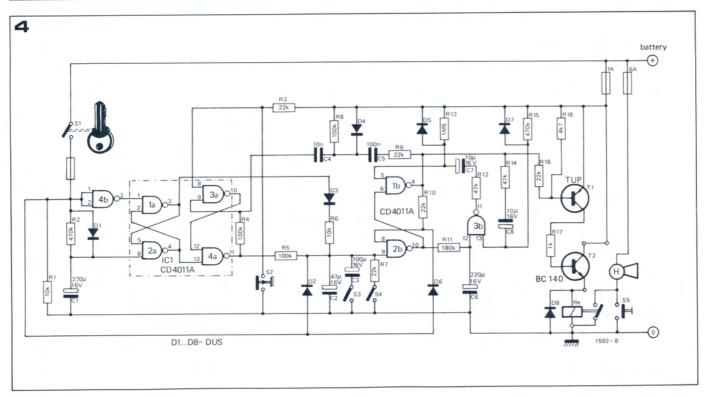
$S_4$  may be a trembler switch or switch(es) on glove compartment, boot etc., which will discharge C2 and C3 rapidly and trigger the alarm.
