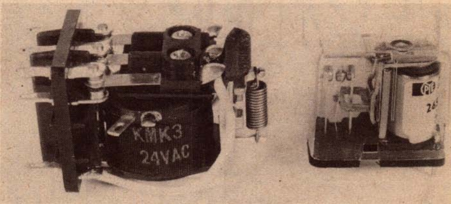
Two relays suitable for the alarm. At left is the "Keyswitch" KMK3 and at right the "Pye" 265. The "Keyswitch" mounts with a single screw, while the author suggests that the "Pye" may be laid flat and glued directly to the board.
