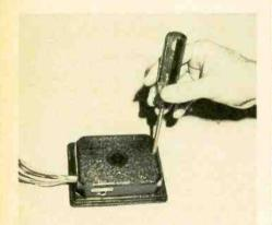
The system boasts a built-in motion detector that will detect a thief tampering with your boat or trailer. Motion detector sensitivity is set by adjusting a small screw found at the top of the module.
