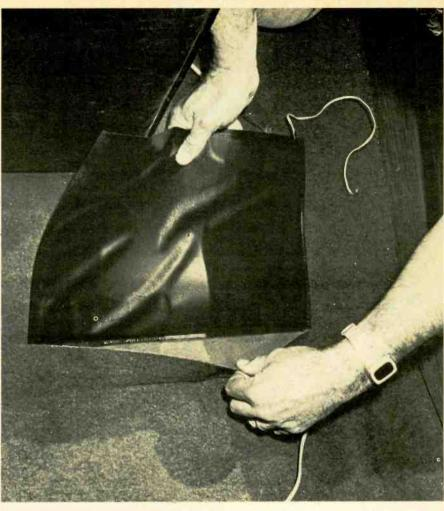
If your boat's carpeting can be pulled up easily, then perform this task and slip the mats underneath. If not, you'll have to slit the carpet with a utility knife for access. Pull back the edge of the carpeting and slide each mat underneath, leaving the wire leads exposed.
