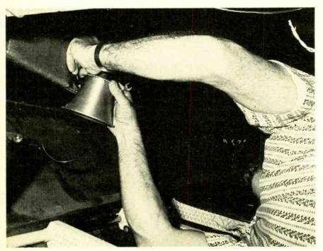
Under the deck, find a suitable mounting spot to attach the horn bracket. Hord the bracket in place, mark through the bracket holes, and drill. Secure the horn to its bracket with hardware provided, then run horn wiring to the alarm module. After all connections are made per directions the system is ready to work for you to protect your investment.
