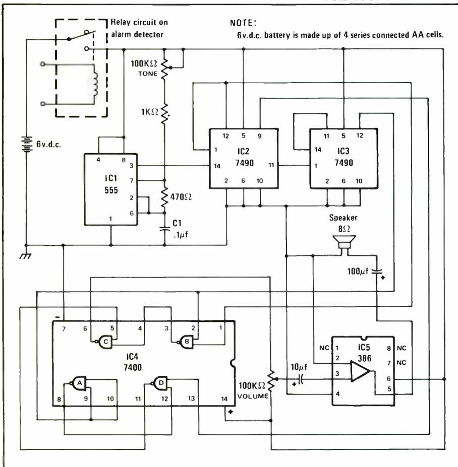
If you'd prefer, you can power it from the alarm detection power supply. However, because the circuit uses TTL integrated circuits, you must meet the exact five-volt TTL voltage rating. If you don't, the ICs will self-destruct.
