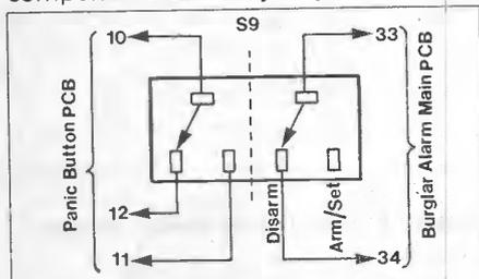
Figure 3. Keyswitch connections
