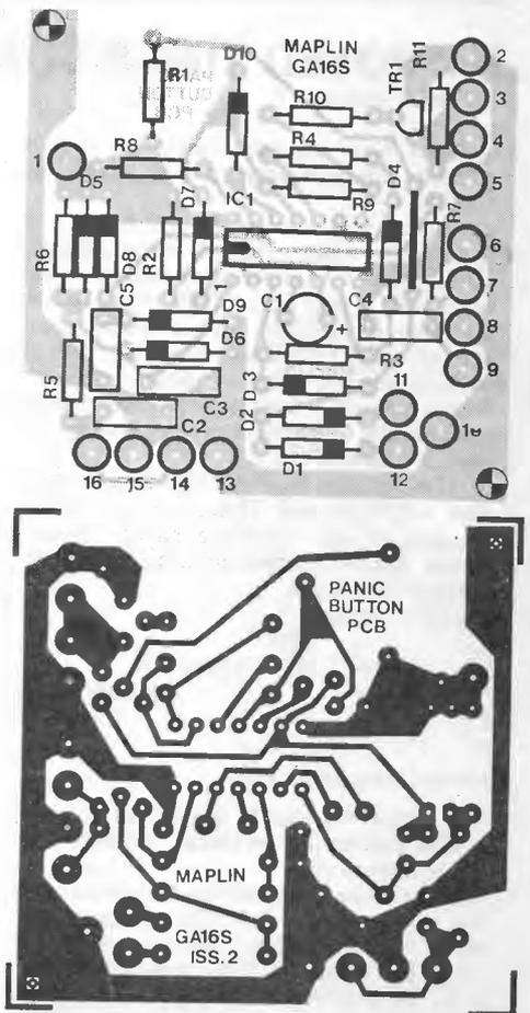
Figure 2. PCB layout and legend
