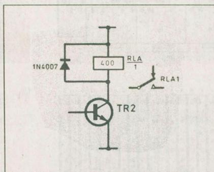
Fig. 2. Addition of a relay to drive other output devices.
