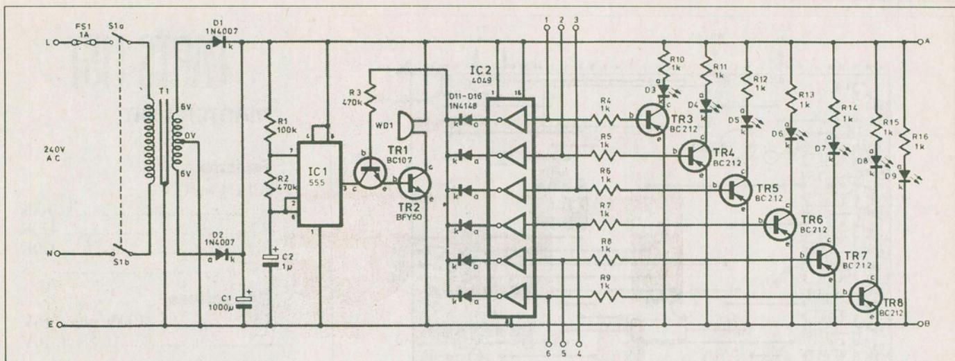
Fig. 1. Circuit of the Fire Alarm master unit.
