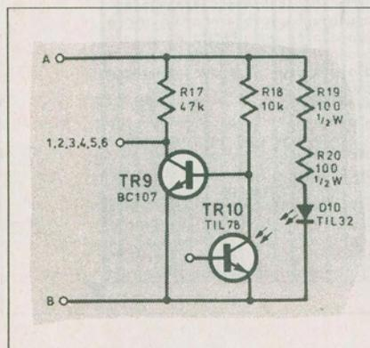
Fig. 3. Circuit of the alarm detector.
