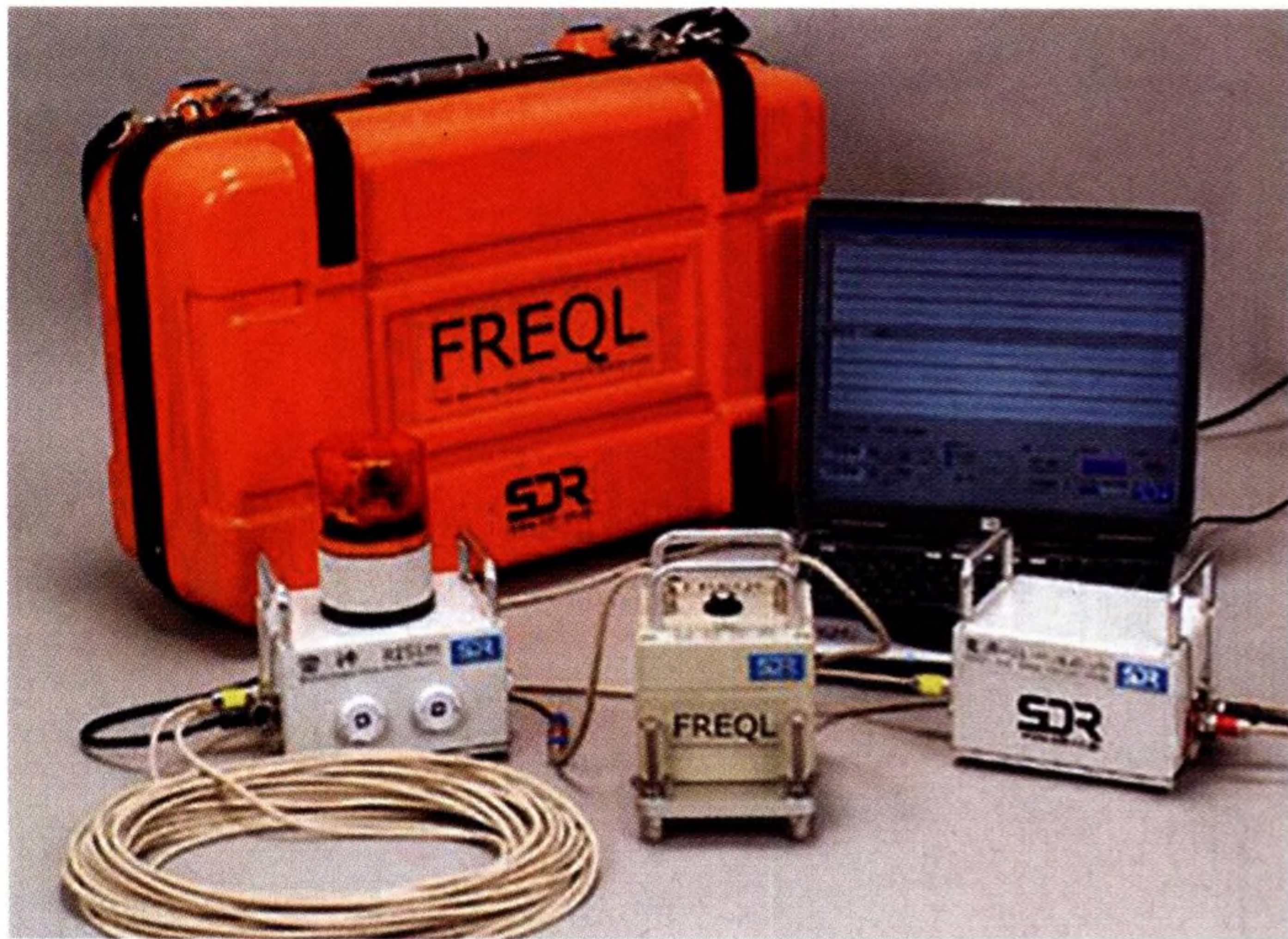
A commercial earthquake early warning alarm, the FREQL (Fast Response Equipment against Quake Load), used by rescue teams in earthquake areas. Ours is very much simpler . . . and cheaper!
